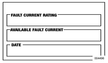
Figure 3-10. Fault Current Label
