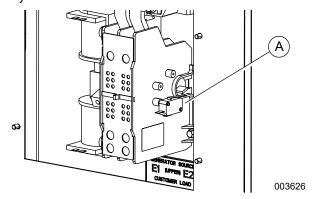
Figure 3-9. Auxiliary Contact
