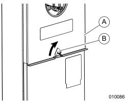
Figure 3-1. Rotate Latch
