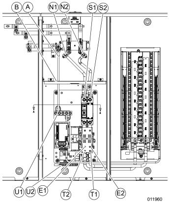
Figure 3-7. Wiring Connections
