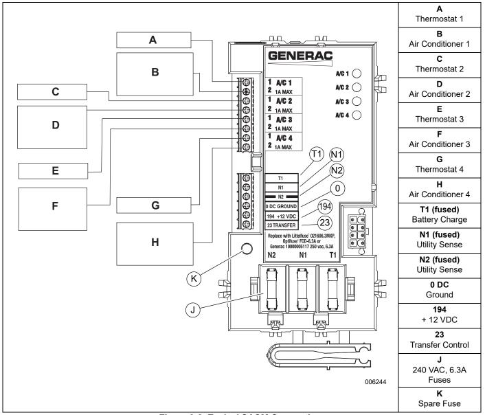
Figure 3-8. Typical SACM Connections
