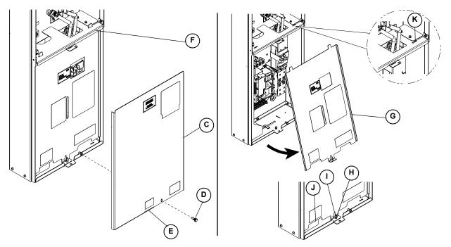
Figure 3-3. Remove Bottom Cover and Panel (ATS)
