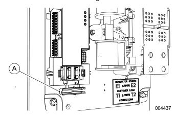
Figure 4-2. Fuse Removal and Installation Tool
